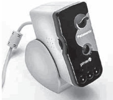
Figure 1-1 The Panasonic DT120 is a small iris scanner for desktop computers.
