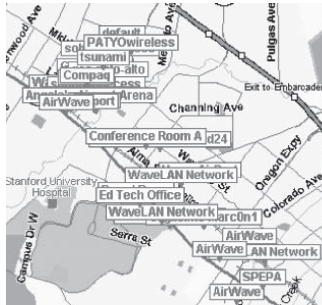
Figure 5-18 NetStumbler can generate street maps of detected access points.
