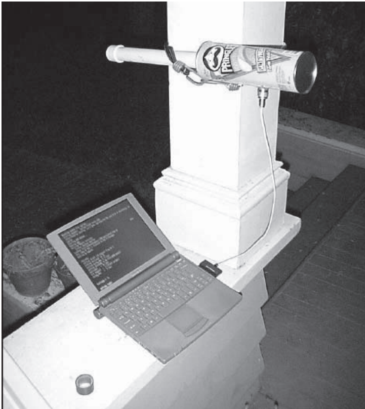
Figure 5-16 A Pringles can makes a decent antenna.
