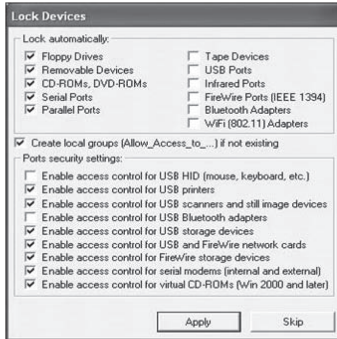
Figure 1-2 DeviceLock can automatically lock devices.
