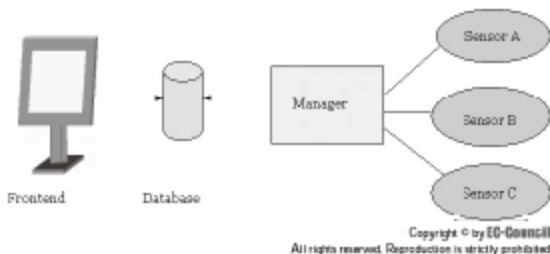
Figure 4-14 This diagram shows the interaction between Prelude components.
