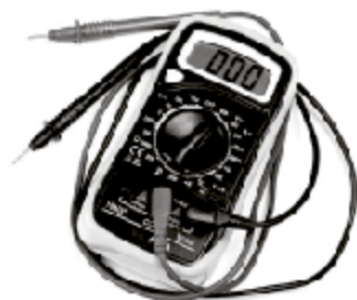
Figure 5-11 A voltmeter measures the potential electrical difference between two points in an electric circuit.
