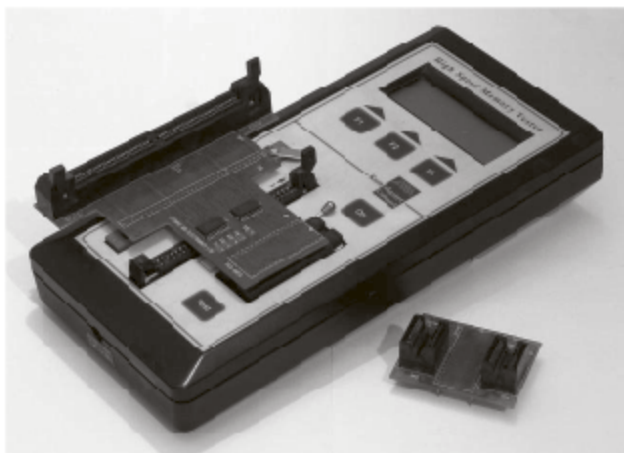
Figure 5-7 A memory tester makes it easy to determine if memory works.
