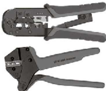
Figure 5-8 Wire crimpers tighten crimps to make permanent electrical connections.
