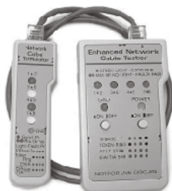
Figure 5-12 A cable tester can diagnose bad cabling and connectors.
