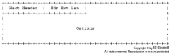
Figure 3-12 This is the format of the hop-by-hop option field.
