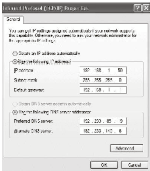
Figure 1-4 Static addressing can be performed through the Control Panel.
