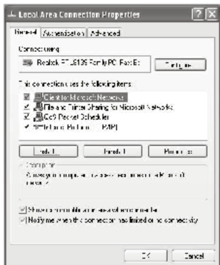
Figure 2-10 Click the Install button in the Local Area Connection Properties window.
