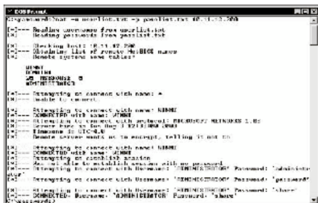
Figure 2-1 The NetBIOS Auditing Tool (NAT) can be used to extract passwords.
