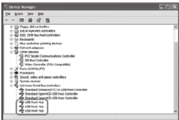
Figure 8-2 These active USB root hubs will connect external USB drives to the system.
