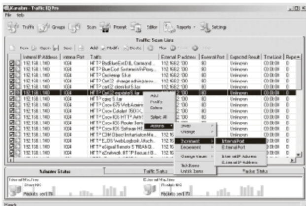
Figure 4-7 Traffic IQ Professional generates traffic between two virtual machines to test security systems.
