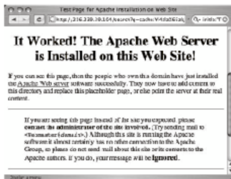
Figure 1-48 Default Web pages for servers can indicate a poorly maintained system.
